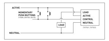
Figure 1. Normal wiring diagram
