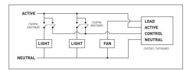
Figure 3. Fan delay timer with multiple lights
