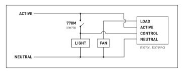
Figure 2. Fan delay timer
